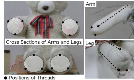
Fig. 4 Positions of the Threads of the Arms and Legs
