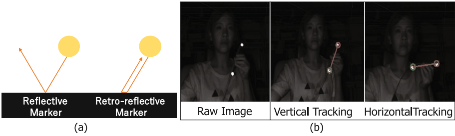
Fig. 5. (a) Property of retro-reflective marker (b) Raw image captured from Kinect IR camera (left), and tracking result (middle and right)
